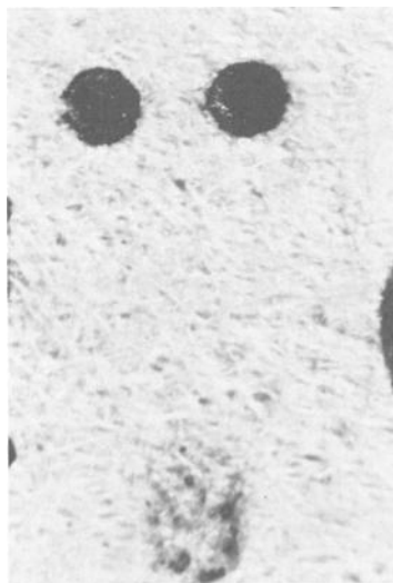
FIG. 6— The mark appearing under the umlaut is due to extensive hammer pressure on the printer causing the lower portion of the backpad to bend forward and strike the ribbon.
