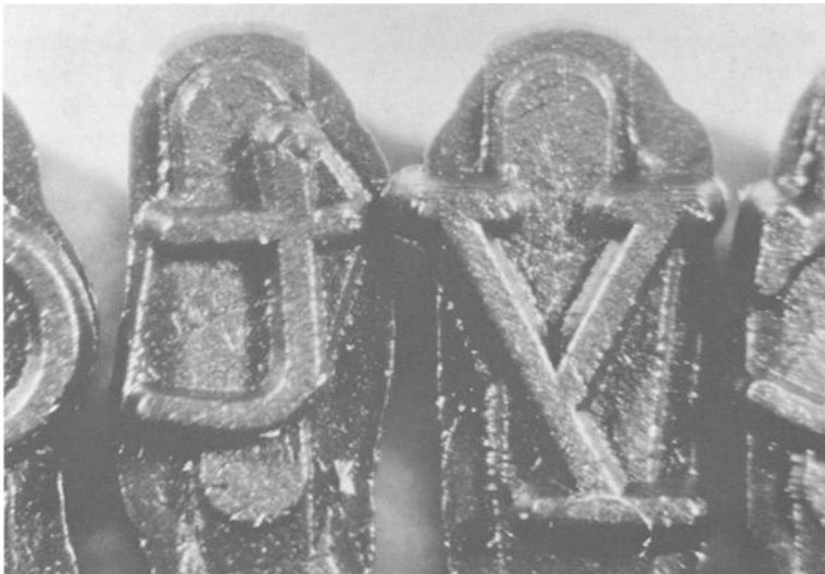
FIG. 1—The “t” and “y” spokes on this printwheel were molded together by excess plastic that escaped from the mold cavities as a result of warpage of the mold. This is a problem indicative of the use of soft molds.
