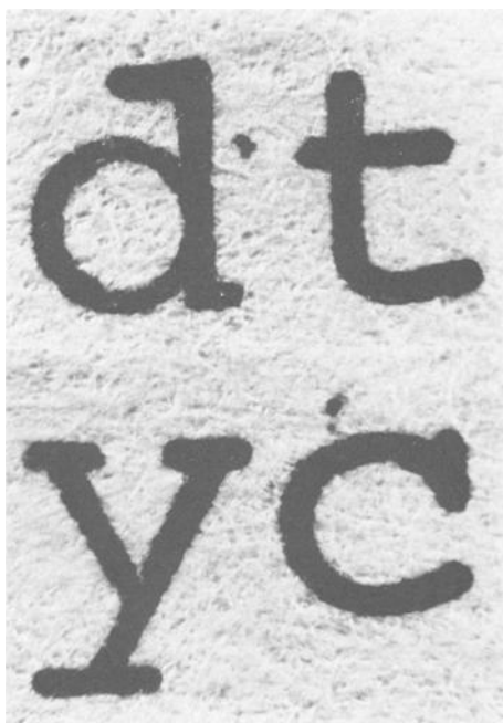
FIG. 7—The marks appearing to the left of the "t" and above the "c" are artifacts caused by the bonding of the two spokes illustrated in Fig. 1.
